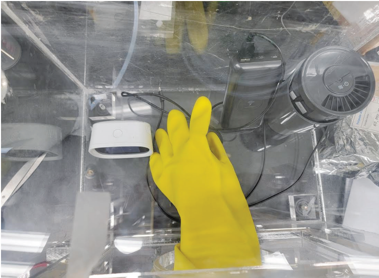
The AP system has a sensor (left), an air purifier (right), a power bank, and a glove. [Source: Author, Charis Kim]
